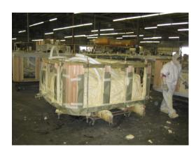
As you would have seen from the previous images there is a lot of pipework around the spa and this has a large surface area that will radiate heat so unlike most manufacturers we foam all of the pipework on the spa to keep the heat in and save on running costs. It also gives added protection and strength.
