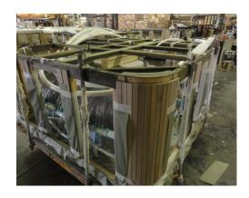
The spa structural timber is all pressure treated and levels checked and adjusted. When the cabinet is fitted the exposed sections are protected before the next stage of production applying the insulation
