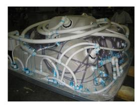
As you will see the plumbing is not for the faint hearted! Blue glue is used so every joint can be visually checked. Some models have over 200 meters of pipework! all this to ensure the client get the most effective bathing and hydrotherapy experience possible.
