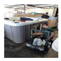
Only after a 73 point check list is completed and signed off by the finishing supervisor is the spa packaged and heat shrink wrapped so the client will receive it in perfect condition
